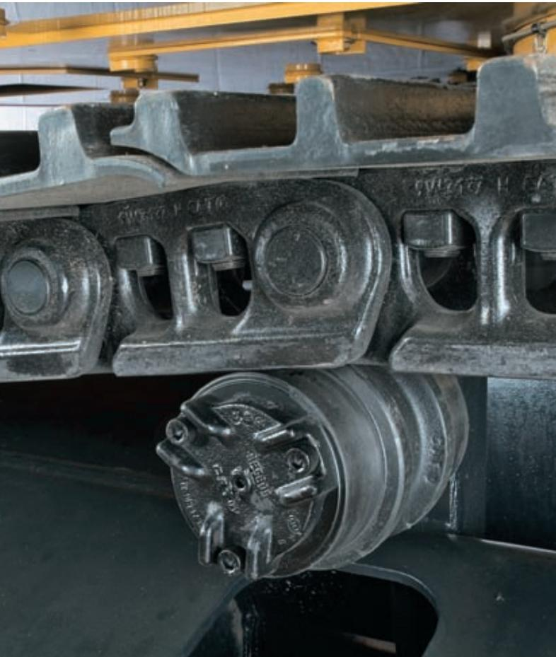
Caterpillar uses advanced engineering and software to analyze all structures, creating a durable, reliable machine for the toughest applications. More than 70 percent of the structural welds are robotic and achieve over three times the penetration of manual welds. These structural components and the undercarriage are the backbone of the machine's durability. The 319D L undercarriage is extremely durable and integrates parts of larger excavators.
